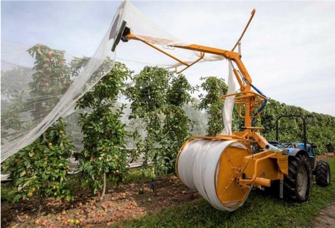
A drape net machine erecting orchard netting at Tulpieskraal.
