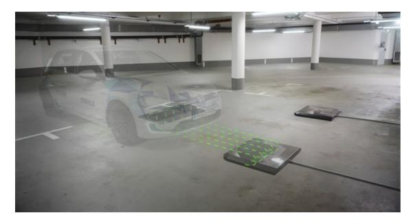
DIPS system represents a shift in e-mobility, offering a convenient alternative to traditional charging methods. It utilises a magnetic field to automatically connect the electric vehicle with the charging point as it approaches. A specialised navigation system in the vehicle display assists the driver in positioning the car optimally for charging.
