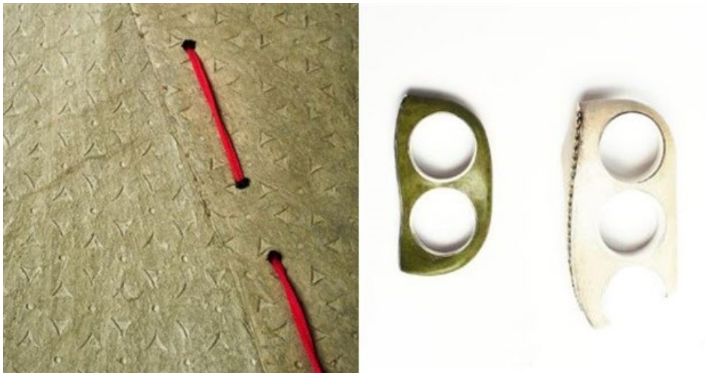
(Left) Hester Erasmus, PPC Imaginarium finalist: high performance Portland cement, latex additives and rubberised textiles create a flexible cementitious material for fashion applications. (Right) Mgnon Dauberman, PPC Imaginarium finalist: using chemical stains, microscopic scale silica aggregates and macrosynthetic fibres pushes the boundary of concrete as a jewellery manufacturing material.
