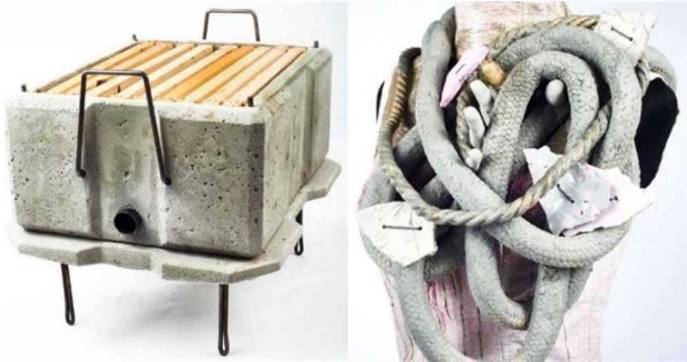
(Left) Ivan Brown, FPC Imaginarium finalist, experiments with additives and alternative materials including aggregates creating a new lightweight insulating concrete. This was used to create a concrete beehive which is fire and termite resistant, thermally stable and cheaper to produce than traditional timber hives. (Right) Meke Vermeulen, FPC Imaginarium finalist, combines traditional Portland cement with latex-based additives and rope fibres allowing new aesthetic and textile application possibilities.
