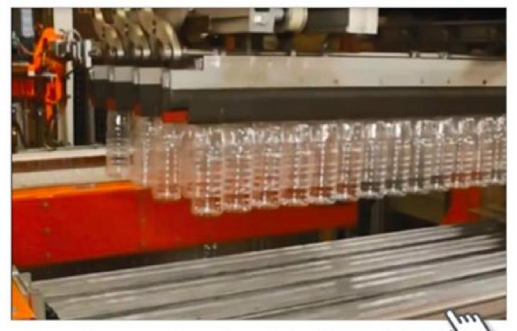
View our two-stage injections stretch blow moulding process here.
