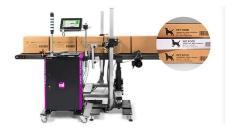
The 5940 G features Markem-Imaje's proprietary Touch Dry inks that instantly dry on contact. This not only increases readability but also offers more reliable traceability. And, unlike liquid inks, Touch Dry inks are ideal for secondary packaging because they don't lose resolution by spreading along corrugated fibres. The inks, which are available in a variety of colours, are VOC-free, safe to handle, and support sustainability.
