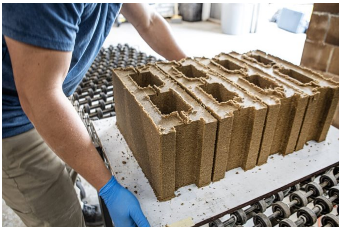
Prometheus Materials' bio-cement is used to form zero-carbon Bio-Blocks on their way to finishing, evaporating and inventory. Source: Prometheus Materials.
